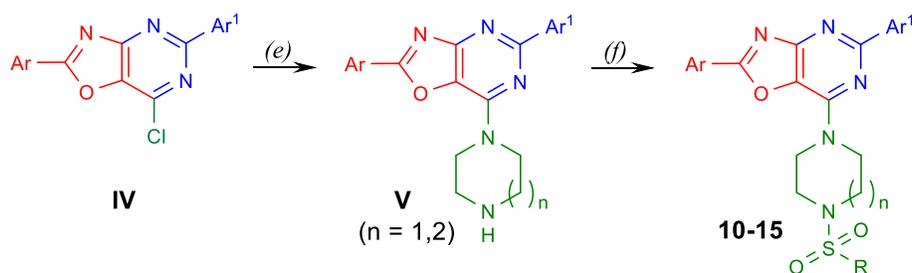
**Scheme 2.** Synthesis of oxazolo[4,5-*d*]pyrimidines **10-15**. Reagents and conditions: (e) piperazine or 1,4-diazepane, dioxane, reflux, 6h; (f) corresponding RSO<sub>2</sub>Cl, Et<sub>3</sub>N, dioxane, 105 – 110 °C, 6h.
