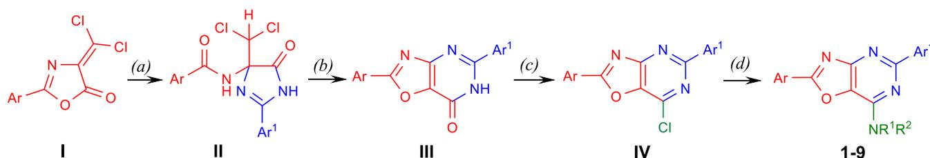
**Scheme 1.** Synthesis of oxazolo[4,5-*d*]pyrimidines **1-15**. Reagents and conditions: (a) amidine hydrochlorides, Et<sub>3</sub>N, THF, r.t., 48h; (b) Py, reflux, 10h; (c) POCl<sub>3</sub>, Me<sub>2</sub>NPh, 105 – 110 °C, 3h; (d) corresponding amine, dioxane, reflux, 6h.
