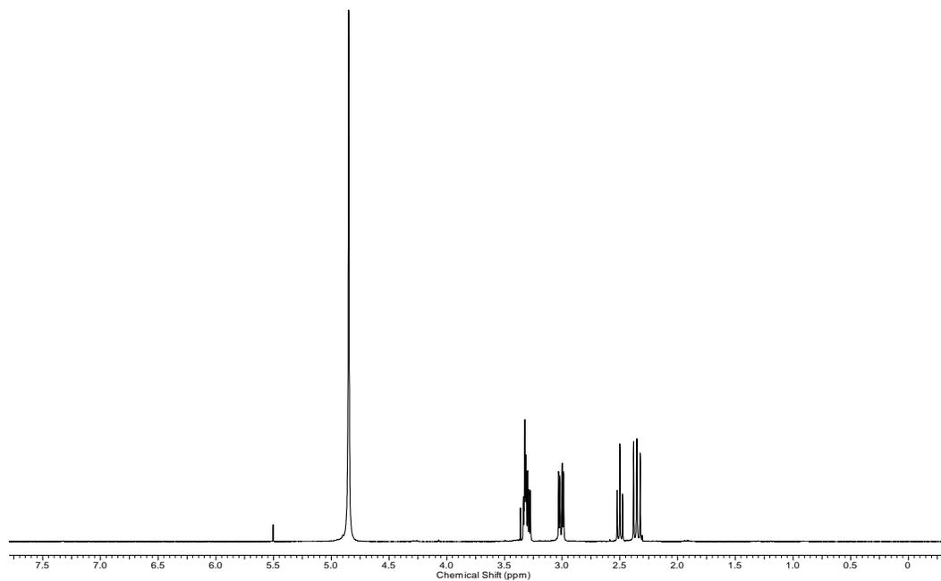
$^1\text{H}$  NMR spectrum (400 MHz,  $\text{CD}_3\text{OD}$ ) of 4-aminopiperidine-3,5-diol (**11**).
