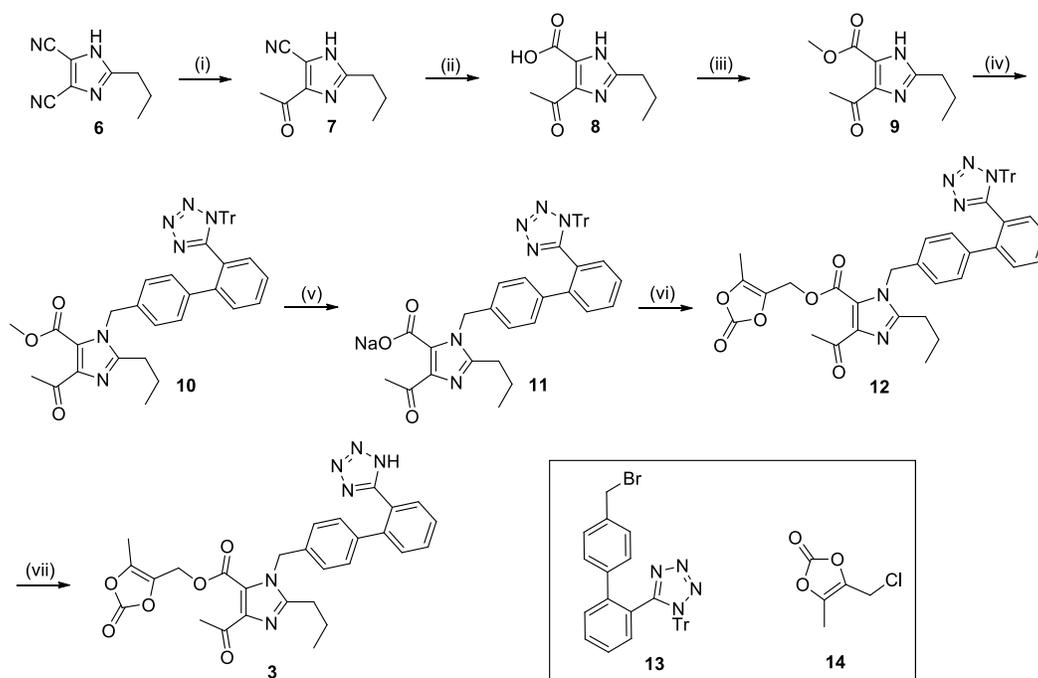
*Reagents and conditions:* (i)  $\text{CH}_3\text{MgCl}$ , THF. (ii) aq. HCl. (iii) Methanol/HCl. (iv) **13**,  $\text{K}_2\text{CO}_3$ , acetone, reflux. (v) NaOH/  $\text{H}_2\text{O}$ /acetone. (vi) **14**,  $\text{NaHCO}_3$ /DMF at 45-50 °C. (vii) Acetic acid/Acetone at 50-60 °C
