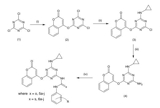
**Scheme 1.** Synthesis of the titled compounds. (i) 4-Hydroxy coumarin, Acetone, Na<sub>2</sub>CO<sub>3 (aq)</sub> (10%), 0-5°C, (ii) Cyclopropylamine, Acetone, Na<sub>2</sub>CO<sub>3 (aq)</sub> (10%), 30-45°C (iii) Ammonia, 1,4-dioxane, 70-80°C (iv) Ar-NCX, Ethanol, reflux.
