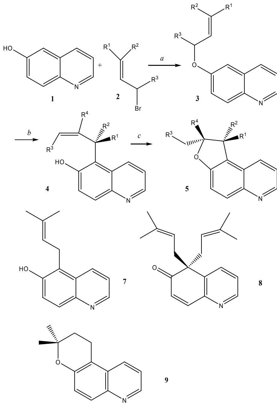
**Scheme 1.** Reagent and conditions: (a) NaH, DME, r.t.; (b) microwave oven, 175°C; or chlorobenzene, reflux; (c) H<sub>2</sub>SO<sub>4</sub>, 100°C.
